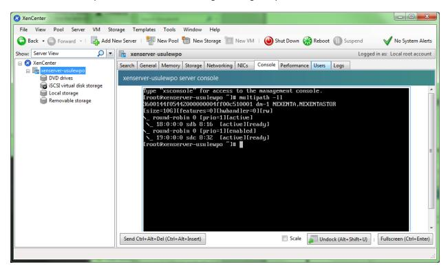
You now have an iSCSI Storage Repository on XenServer 6 that is multipath. Assuming the two IPs in use come from separate NICs on the XenServer and go to separate switching fabris, the storage now is wholly redundant and, in typical use, potentially up to twice as fast.
