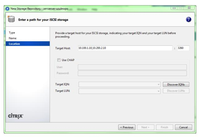
As the picture shows, on this page, type in the IP of the first Target Portal Group from your NexentaStor appliance (as with all other examples in this guide, this is 10.100.1.10 for us), followed by a comma, and then the IP of the second Target Portal Group (10.200.2.10 for this example) and then click the "Discover IQNs" button, which will become clickable after you type in a valid IP in the "Target Host" field.
