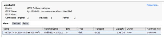
If it does not, open the iSCSI Adapter back up and be sure to add in the proper network adapters to it so that it can pass traffic. Be sure to add all adapters necessary to provide IP connectivity for all the IPs used for the MPIO connection. You may test connectivity from the ESXi host by opening up a SSH session and run the command:
