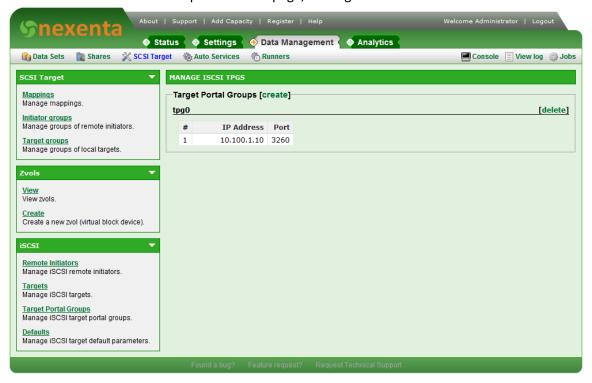
As you can see, the page has changed slightly. Most notably, in addition to listing your new Target Portal Group "tpg0", the "create" link now exists instead of the old "here" link from before. Click the "Create" link and fill in the information again, but this time creating the second TPG with the 10.200.2.10 IP address. Note that the name of a Target Portal Group is entirely unimportant—you can name them
