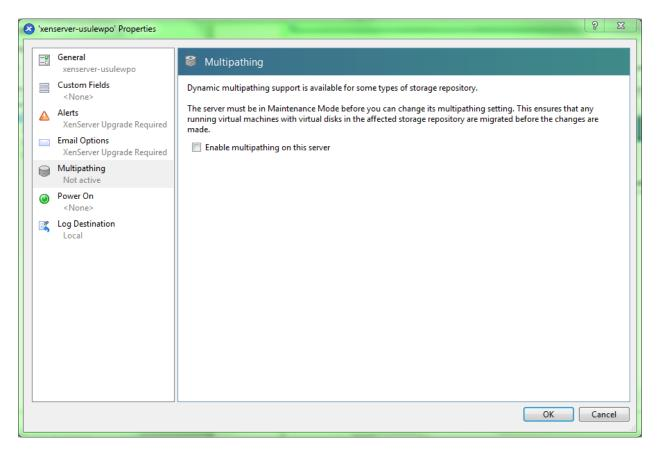
Check the "Enable multipathing on this server" checkbox and hit OK.
