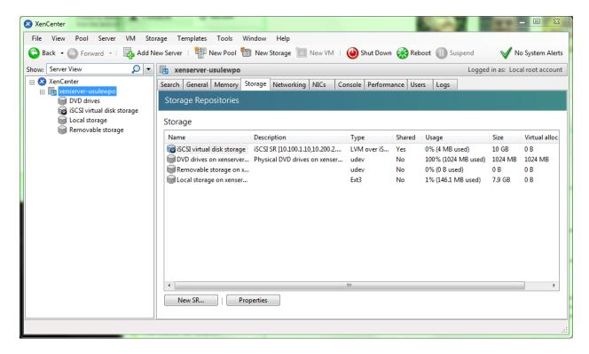
This storage is, by virtue of how it was created, multipathed. One way to quickly verify this is to click the **Console** tab, hit **Enter** to login, and then, at the prompt type "**multipath -II**".
