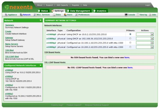
To configure a network interface in the NMV, mouse-over **Settings** and then choose **Network**. On the resulting page, similar to the one pictured above, pick the interface you wish to configure from the list by clicking its interface name (for instance, e1000g2), which will result in this page:
