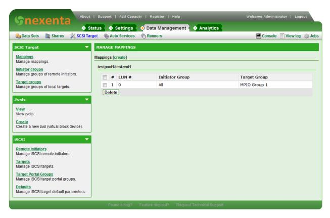
This confirms for us that a new mapping now exists for the testpool1/testzvol1 Zvol, offered up as LUN 0 to any initiator (client) who connects to any of the Targets in "MPIO Group 1".
