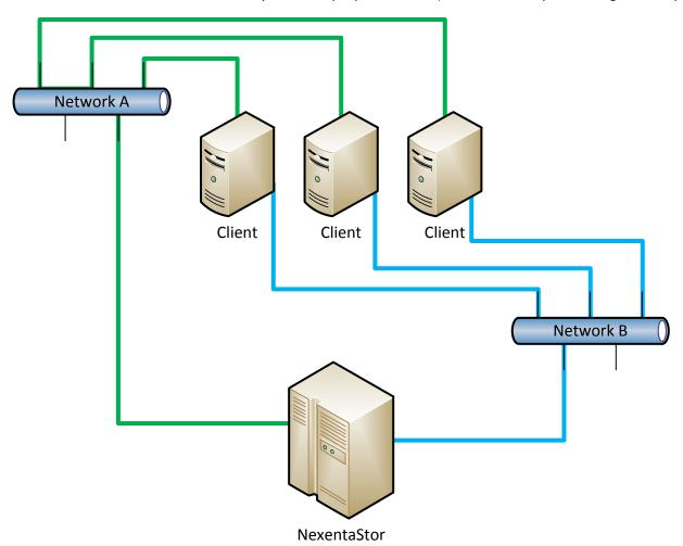
This diagram shows the two separate networks (A & B) connected from each client and NexentaStor; this provides both path redundancy and switch redundancy (assuming there are one or more switches on each network), and may increase performance by as much as double that of a single link.
