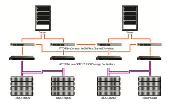
NexentaStor MetroHA combines a synchronous storage solution with ZFS end-to-end data integrity. In the event of a total site disruption, data services are restored at the secondary location or remote site within a matter of seconds.
